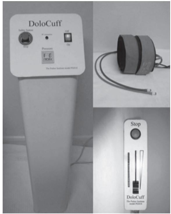
Fig. 1. The computerised cuff pressure algometer (CPA), including compressor and control panel, inflatable cuff, and a stop-button with integrated visual analogue scale.
